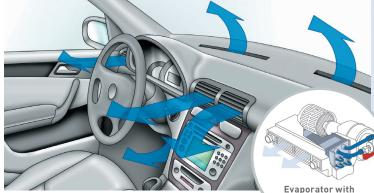
Evaporator with ventilation system
