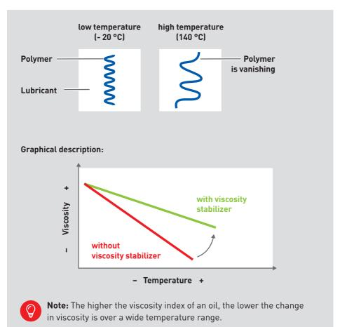
The image shows how this mechanism works:
