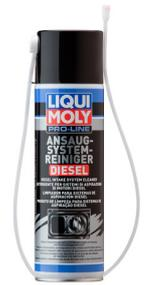
Spray the Diesel Intake System Cleaner into the intake system via the spray probe in short intervals of 2 – 3 seconds at min. 2,000 revolutions. Move the probe back and forth in the process to clean the entire intake tract.
